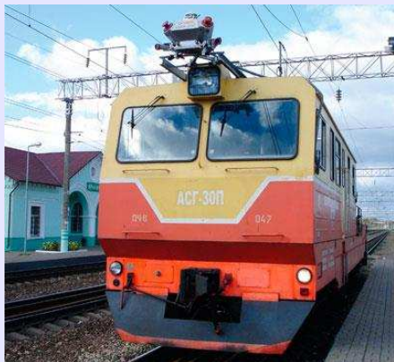
Fig: Laser scanner on train ( http://nipistroytek.ru/ ).
